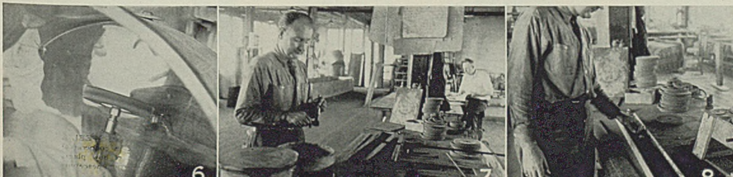
Fig. 8—Abrasive is applied to the wheel after brushing with binder by rolling in a trough containing the abrasive material. Drying rack can be seen at extreme right
