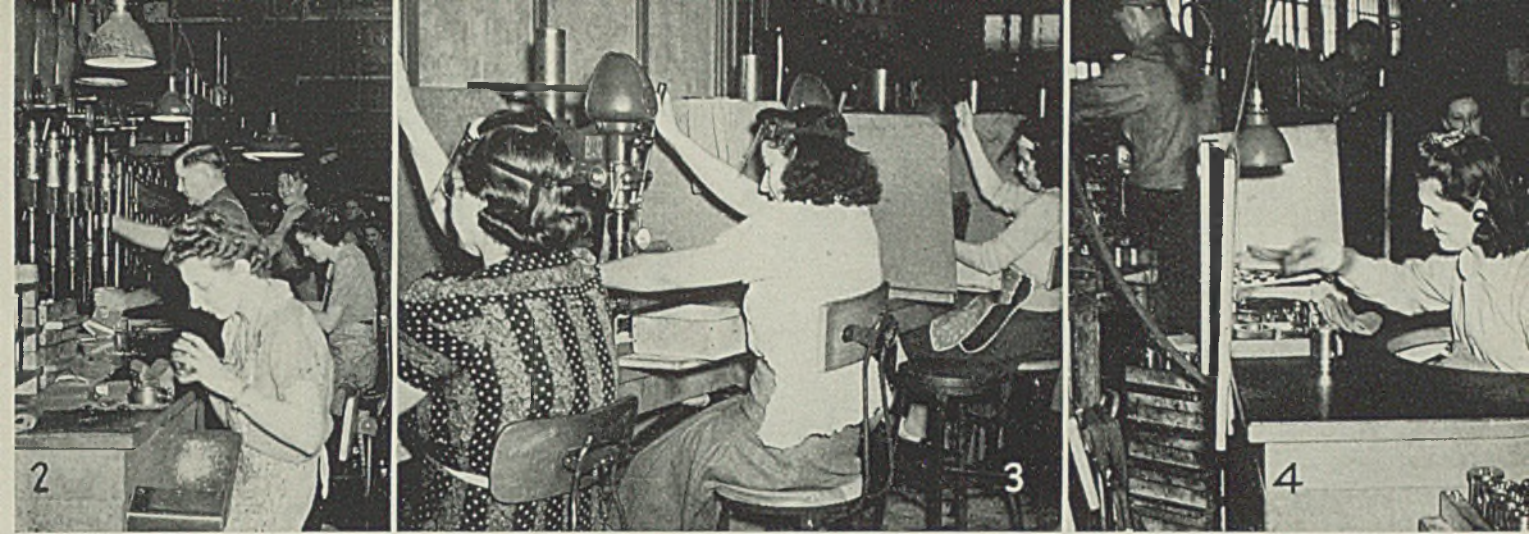
Fig. 1—Simple, medium duty drill presses—both singly and in multiple grouping—are used liberally throughout the plant to handle subdivided secondary operations and to keep larger, more powerful “critical” machine tools clear to cope with the more complicated and heavier operations which only they can handle effectively
