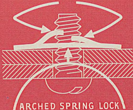
ELIMINATE THREADED NUTS AND LOCK WASHERS
