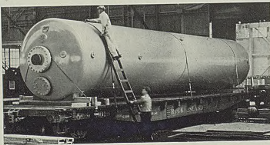
■ The accompanying illustration shows a 45-foot flange steel pressure vessel recently built by Chicago Bridge & Iron Co., 332 South Michigan avenue, Chicago, for the University of Iowa. Designed to house atom-smashing equipment and to withstand pressures of 125 pounds per square inch, this 8½-foot diameter unit is entirely of welded construction, all seams being butt welded and ground smooth on the inside to prevent unnecessary loss of electric potential
