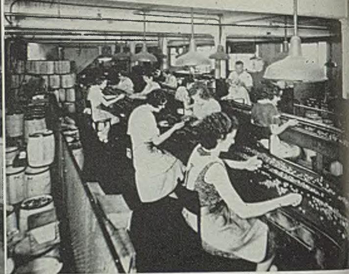
Fig. 1. (Left)—Part of heat-treating department showing electric furnaces, gravity conveyors and automatic overhead cranes. Fig. 2. (Right)—Belt conveyors used for inspection and sorting permit a number of operators to work simultaneously to take care of a large belt load easily
