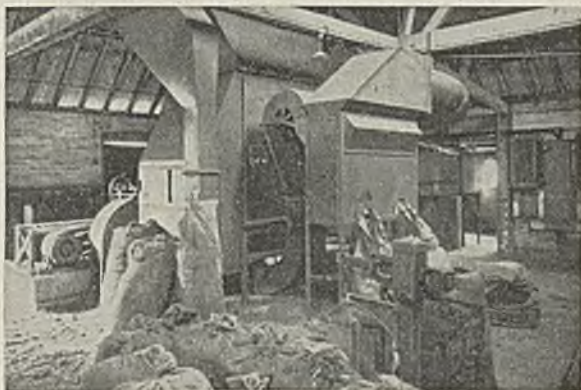
General view of dryer, showing winnowing equipment and dry grain discharge to bags
