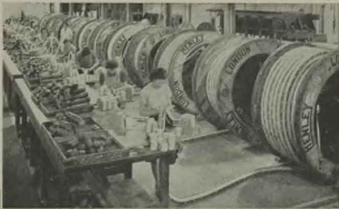
Assembling buoyant cable centres and (left) the component parts comprising inflated rubber elements, wood reinforcing discs and longitudinal strengthening tapes
