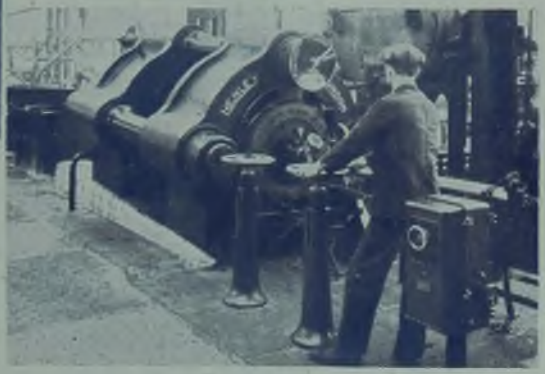
Coiling a length of many miles of H.A.I.S. Cable outside the HENLEY Cable Factory to await shipment.
