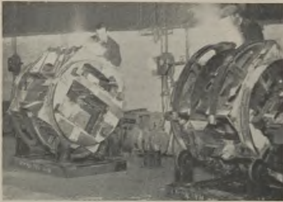
All-welded steel cradle for two-pounder pom-poms in course of manufacture
