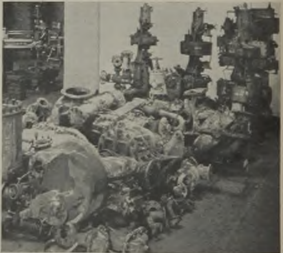
A typical collection of pumps and other machinery from the damaged engine-room of one of H.M. ships, as received for repair
