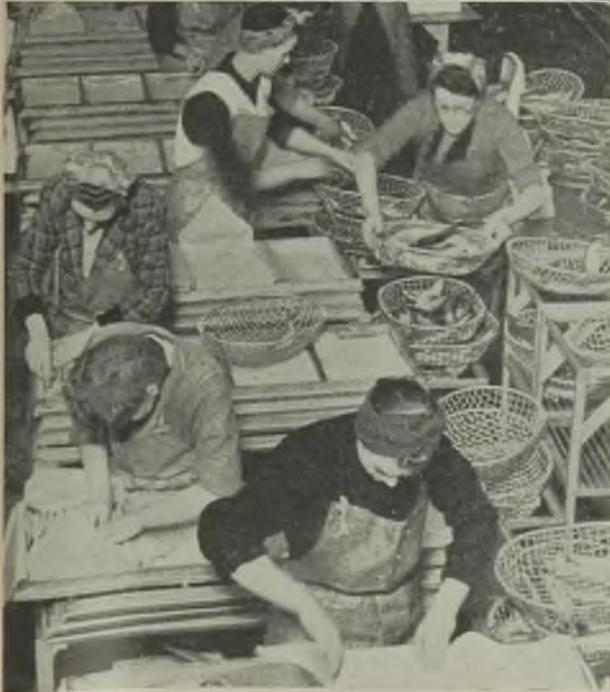
(roughly twenty-three fish). Packers lay the fish neatly in flat aluminium trays containing four 7-lb. divisions, each being separately wrapped in waxed paper. The trays are loaded on to rack trolleys, holding thirty trays, and wheeled to the frosters, of which there are eight, each holding forty-five trays (90 stone).
