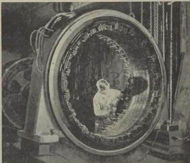
**STATOR OF AUTO-SYNCHRONOUS MOTOR
