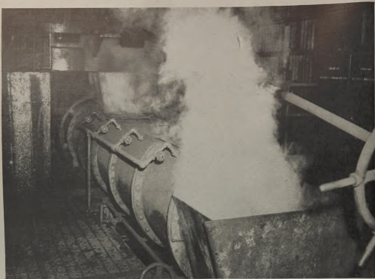
Conditioning equipment ahead of the briquetting press includes this horizontal fluxer.
