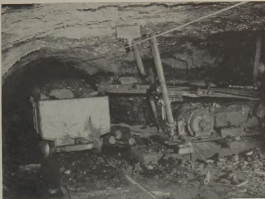
Conveyors discharge directly to the mine cars—in this case a new steel unit.
