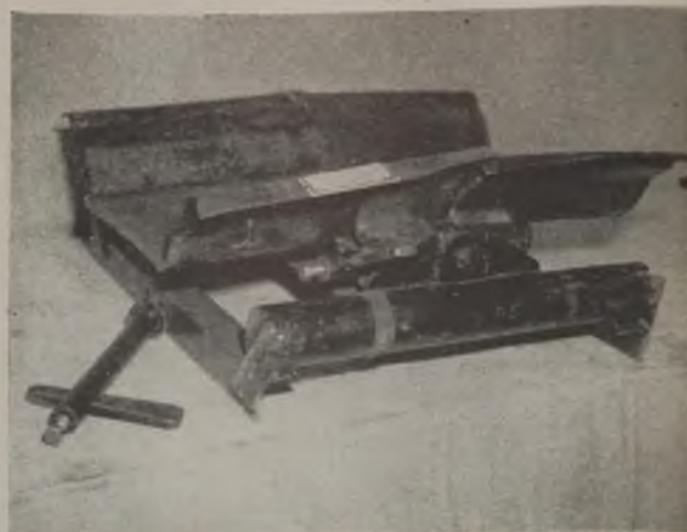
Showing use of wedge-bolt pan fastener.
