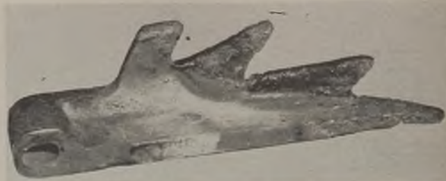
Fig. 2—The badly worn loading-machine arm at the left was rebuilt in six hours with oxyacetylene-welding equipment using about 6 lb. of chrome-vanadium-steel welding rod.
