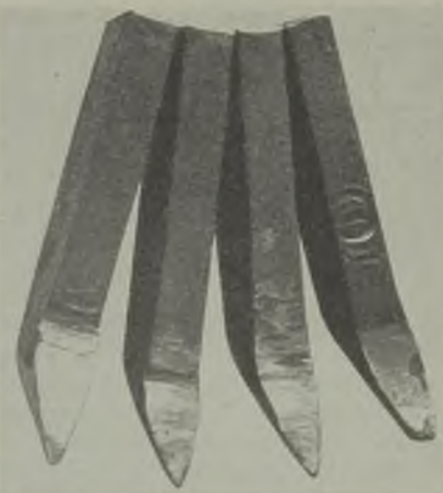
Fig. 8—Hard-facing cutter bits. The jig (left) permits adjacent bits to be preheated while one bit is being hard-faced. Up to 200 bits can be hard-faced in an hour with this set-up, a very economical operation. In the illustration at the right, the bit at the left has been machine forged. Center bits have been hard-faced. Hard-faced bit at right will be reground again after service.
