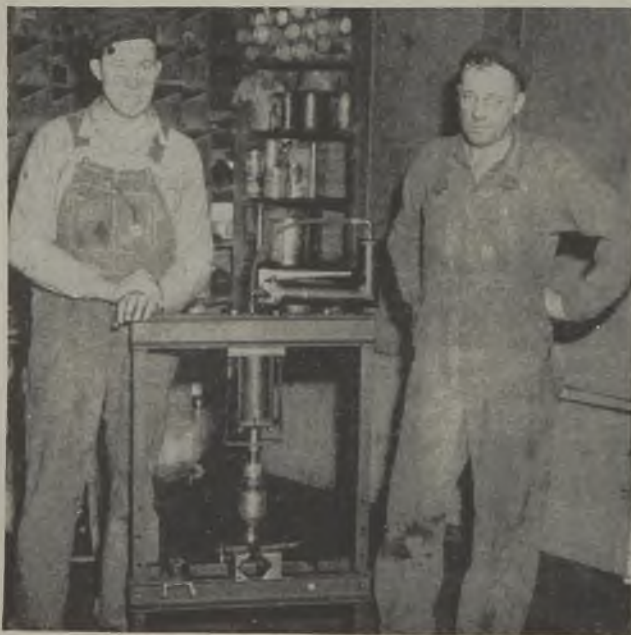
The grease gun powering this small shop-made press is mounted on top of the frame. Messrs. Harris (left) and Middleton pose with their creation.
