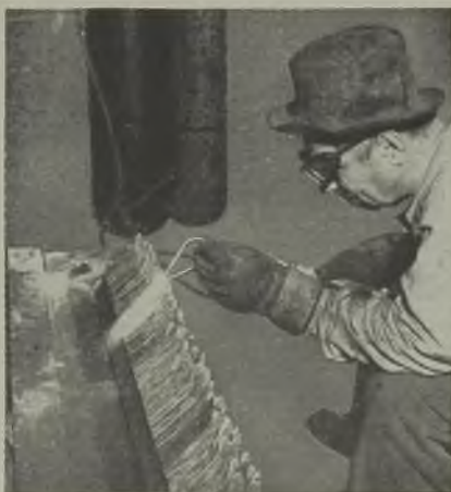
Fig. 8—Hard-facing cutter bits. The jig (left) permits adjacent bits to be preheated while one bit is being hard-faced. Up to 200 bits can be hard-faced in an hour with this set-up, a very economical operation. In the illustration at the right, the bit at the left has been machine forged. Center bits have been hard-faced. Hard-faced bit at right will be reground again after service.
