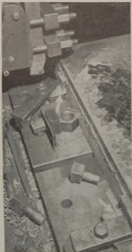
Two clips at each end of the plate make it possible to keep the clamps, which secure the plate to the bed of the planer, well in the clear.
