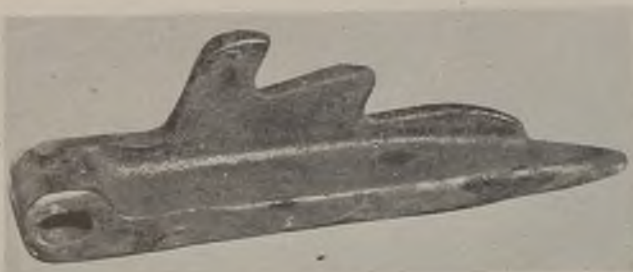
Fig. 2—The badly worn loading-machine arm at the left was rebuilt in six hours with oxyacetylene-welding equipment using about 6 lb. of chrome-vanadium-steel welding rod.
