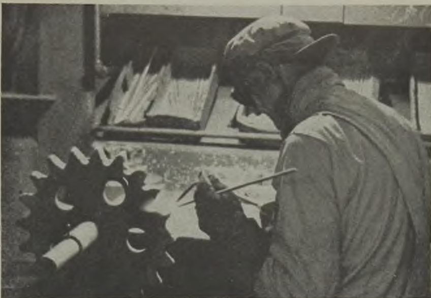
Fig. 7—Hard-facing worn crawler-drive sprocket wheel for loading machine.
