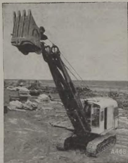
A-468. 2 yd. Amsco All-Manganese Steel Welded Type Dipper on Lorain "82" shovel; used for handling coral rock in New Guinea.
