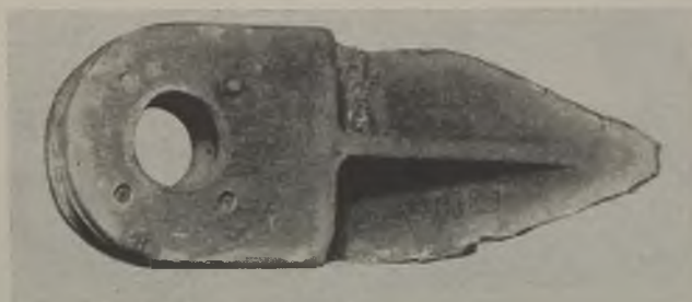
Fig. 3—Reclaimed cast-steel forks for loading-machine conveyor pans wear 20-percent longer than the original when rebuilt with arc-welding equipment. Welding time was 1½ hours on this job. Note the wear in the bore on the fork at the left.
