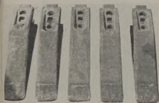
Fig. 10—New hard-faced shovel teeth last two to six times longer than untreated teeth. Periodic building up keeps teeth sharp, increasing tonnage stripped with less power.
