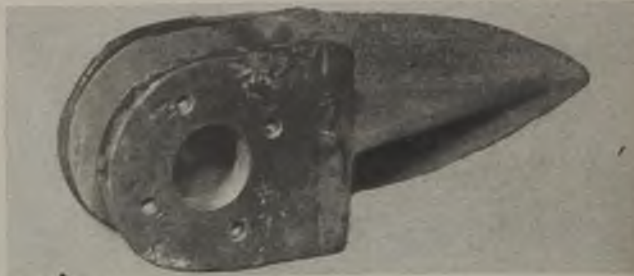
Fig. 3—Reclaimed cast-steel forks for loading-machine conveyor pans wear 20-percent longer than the original when rebuilt with arc-welding equipment. Welding time was 1½ hours on this job. Note the wear in the bore on the fork at the left.
