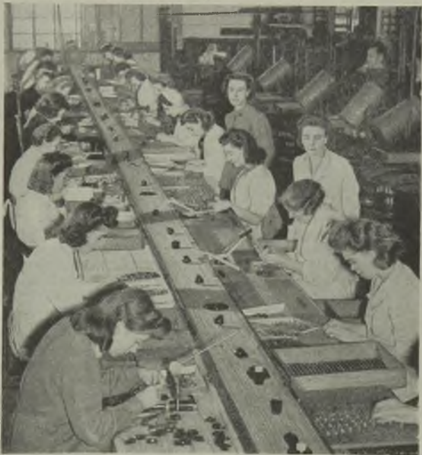
Final assembly conveyor. Note the arms on the edge diverting articles to operators along the line
