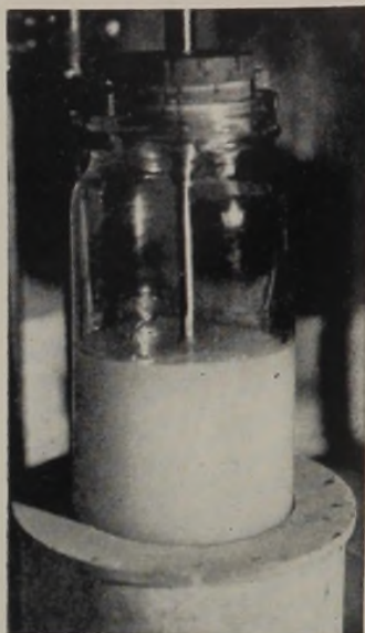
FIG. 4. PREPARATION OF ALUMINIUM STEARATE GEL: GELATION BEGINS.
