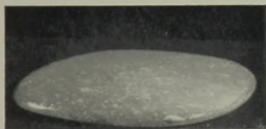
FIG. 12. VISCIOUS FLOW OF SEMI-SOLID GEL : AFTER 2 HOURS.
