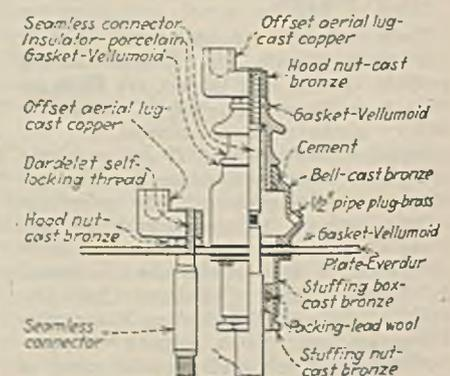
This suspension and terminal unit includes an insulation seal for the positive cable
