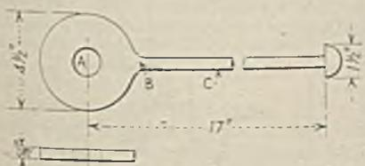
Fig. 8—Showing construction of stop member
