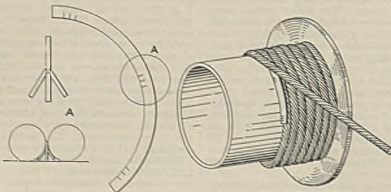
Fig. 2—Left, details of shim; right, method of applying shim in spooling on first wrap on drum
