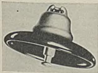
tion is said to increase resistance to breakage in transportation. Mechanical values are the same as the regular O-B 15,000-lb. suspension insulators, as are dry flashover values. Wet flashover values, however, are slightly lower, due to the absence of petticoats. The new insulators are furnished with 10-in. disks in both 5- and 5½-in. spacing, the latter with either ball-socket or clevis attachment. The 5-in.-spaced unit is available with only the ball-socket attachment.
