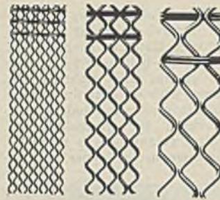
vides enough play so that jammed grains will work themselves out of the mesh without difficulty. Large increases in screen capacity are noted by the company, which is offering the "Snake-Screen" in a number of wire diameters and openings.
