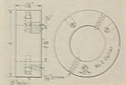
Fig. 5—Details of adjustable collar for use on mandrel
