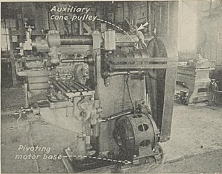
Individual drive applied to machine tool in Union Pacific machine shop. Lever and toggle used to raise and lower the auxiliary cone pulley is indicated by arrow
