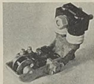
mounting blocks, it is stated, were designed to simplify mounting of brush holders and to locate brushes properly in the correct neutral position.
