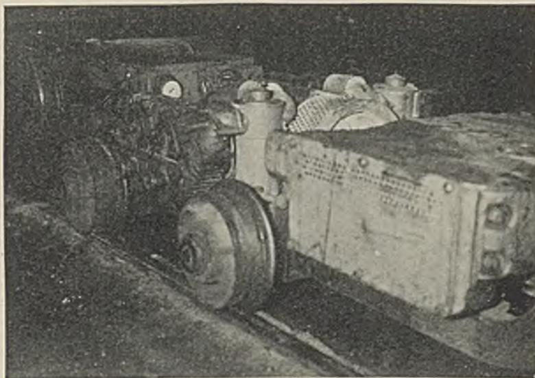
Capacity, 120 cu.ft.; height, 26 in.; and the wheels have 1 in. of vertical play to insure better tracking
