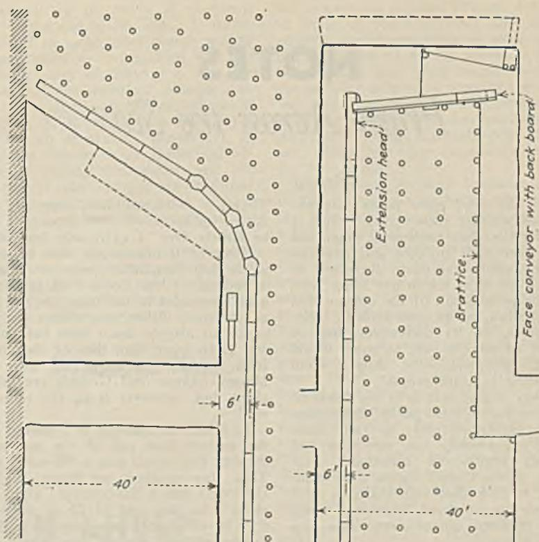
Fig. 2—Left, method of mining pillars open-ended; right, details of room operation, showing how face conveyor is moved up with cutting machine
