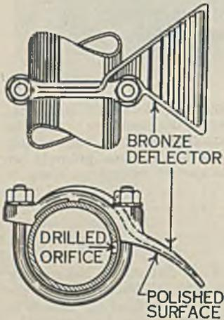
Deflector width permits a comparatively large water jet and thus allows fairly large particles of dirt to pass the orifice without clogging.
