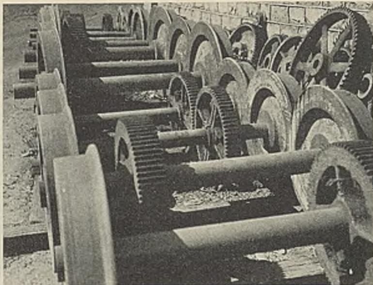
Twenty-three years of experience is back of this assembly of rolled-steel wheels at the Minden shop
