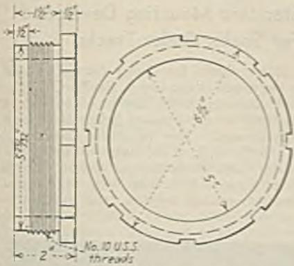
Fig. 6—Construction details of packing nut
