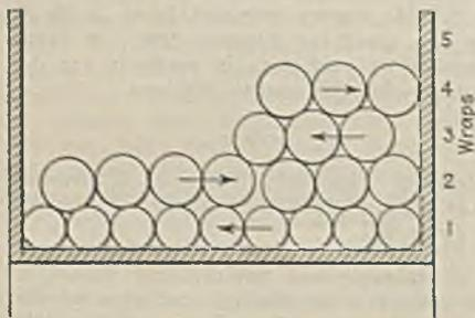
Fig. 1—Diagrammatic sketch (rope size exaggerated) showing effect of decreased rope diameter on spooling when shims are not used
