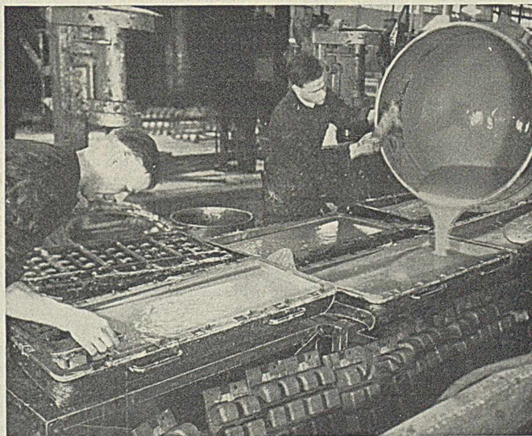
FIGURE 10. POURING COMPOUNDED LATEX FROTH INTO MOLDS DURING MANUFACTURE OF CELLULAR AIR CUSHIONS
