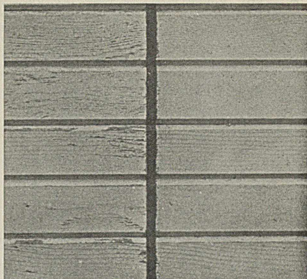
FIGURE 3. EFFECT OF ALUMINUM PRIMING IN RETARDING FLAKING OF LEAD AND ZINC PAINT ON DOUGLAS FIR
