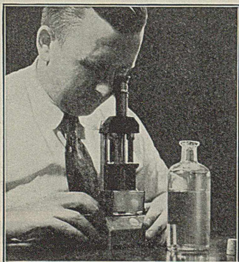
The colorimeter is one of the instruments Rossville uses to assure uniform color and clarity.
