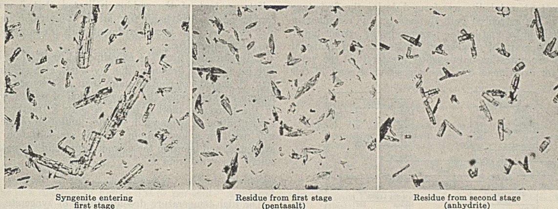
FIGURE 4. PHOTOMICROGRAPHIC COMPARISON OF SOLIDS AT DIFFERENT POINTS DURING TWO-STAGE EXTRACTION OF SYNGENITE AT 200° C. (X 170)
