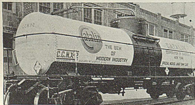
One of the special Nickel-Clad Steel tank cars owned by the American Catalin Corporation, 230 Park Avenue, New York City, for the purpose of shipping phenol. Cars, built by General American Tank Car Co., have 60,000 lbs. capacity and are provided with Nickel coils at bottom for heating.
