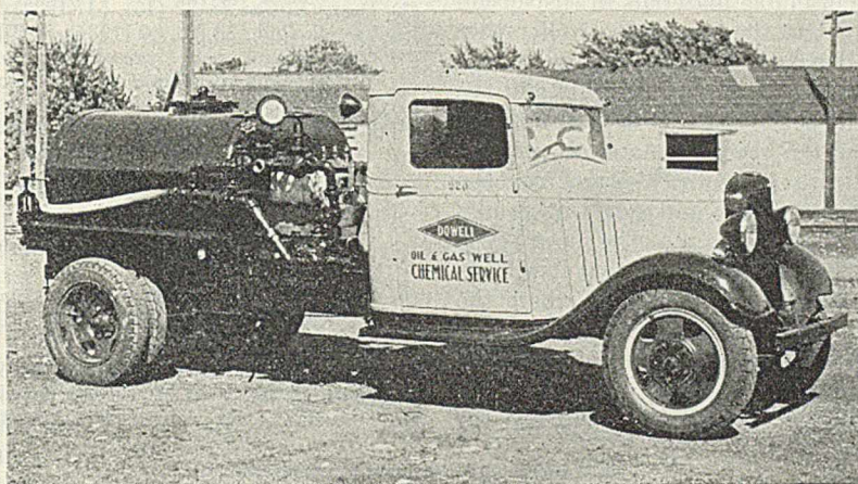
SMALL TRUCK EQUIPPED WITH 500-GALLON TANK AND HIGH-PRESSURE PUMP
