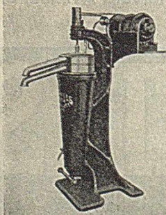
Sharples Super Centrifuge, rotating at a speed of 15,000 R. P. M., generates a centrifugal force of over 13,000 times gravity.
