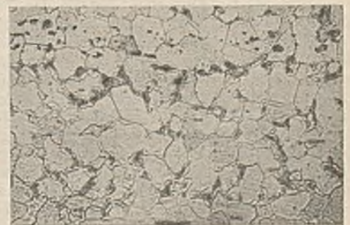
Abb. 4. Korn in der Blechmitte. v. = 150.
