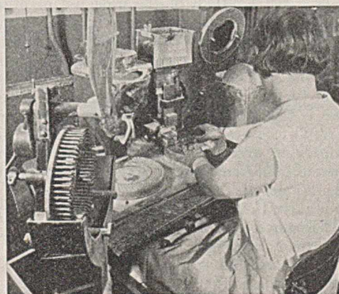
CAPSULE FILLING MACHINE SHOWING FILLING OF EXTRALIN IN LIVER DEPARTMENT, ELI LILLY AND COMPANY
