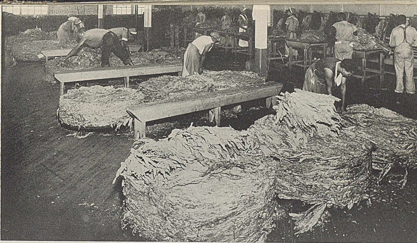
PULLING-UP ROOM WHERE TOBACCO IS REMOVED FROM HOGSHEADS (IN FOREGROUND) AND PLACED IN ORDERING MACHINES (ALONG WALL), WHERE ADDITIONAL MOISTURE IS ACQUIRED
