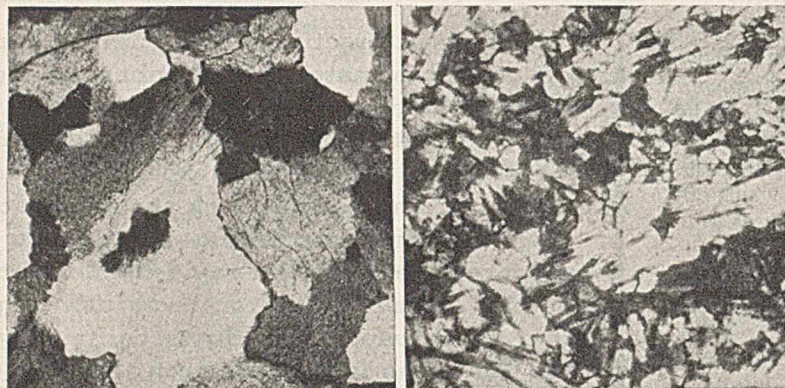
FIGURE 2. PHOTOGRAPH OF THIN SECTIONS OF FUSED PHOSPHATE TAKEN WITH TRANSMITTED LIGHT AND CROSSED NICOLS ( \times 75 )
