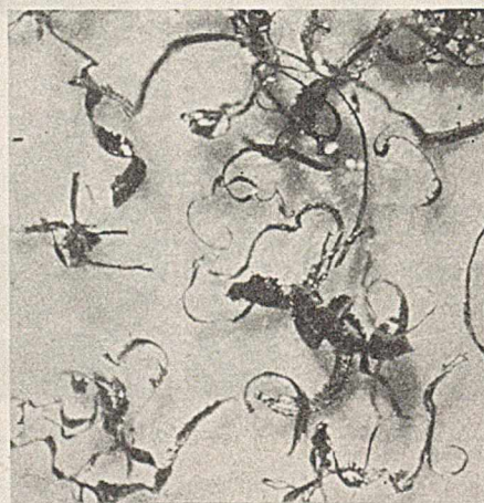
STEEL CHIPS CUT BY A METALITE FIBER COMBINATION DISK (X20)
