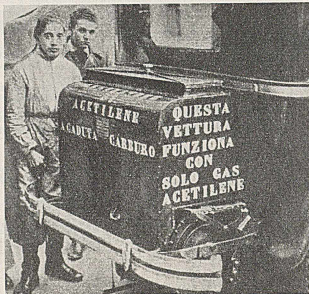
ACETYLENE-BURNING MOTOR CAR, ITALY C 2 H 2 from calcium carbide and water
