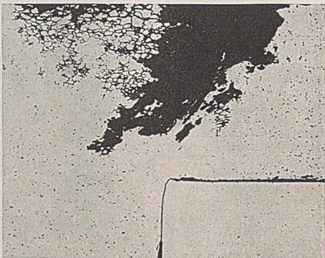
FIGURE 6. INTERGRANULAR CORROSION OF 53ST RIVET IN CONTACT WITH 24ST SHEET ( \times 50 ) (Compare Figure 8B)
