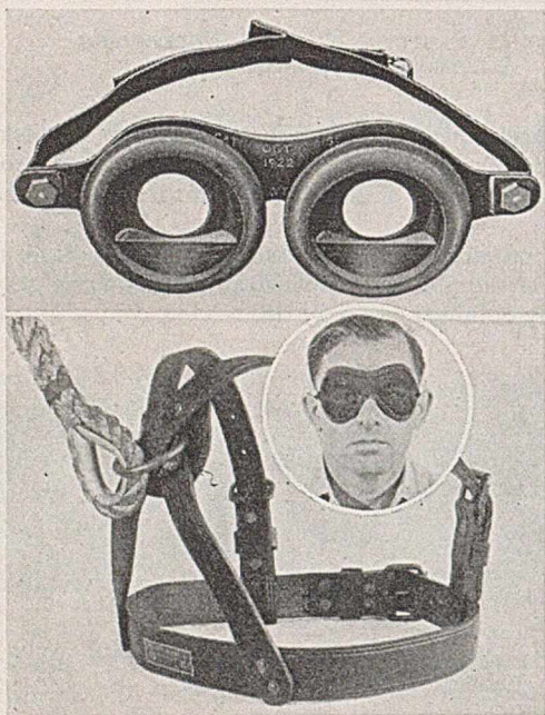
(Top) GASTIGHT GOGGLES FEATURING THE NOD-AND-SHAKE PRINCIPLE BY MEANS OF WHICH THE WATER IN THE CUP OF THE GOGGLES WASHES AWAY THE FOG COLLECTING ON THE LENSES
