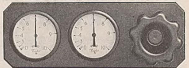
Indicating Receiver (left). Set Pointer (center). Set Point Adjustment (right).
