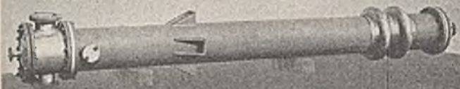
Heat Exchanger, 18" diameter x 16' tube length. Tubes, tube sheets and heads of Aluminum 3S. Carbon steel shell and copper expansion joint.
