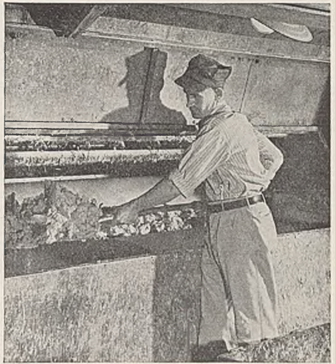
Making GARLOCK 7021 Compressed Asbestos Sheet Packing at the Garlock factory.
