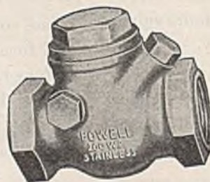
Fig. 1847—200-pound Stainless Steel Swing Check Valve. Screwed ends, screwed-on cap and regrindable, renewable disc.
