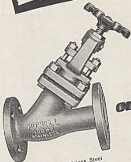
Fig. 2051—150-pound Stainless Steel "Y" Valve. Has flanged ends, bolted flanged yoke, outside screw rising stem and plug type disc.
