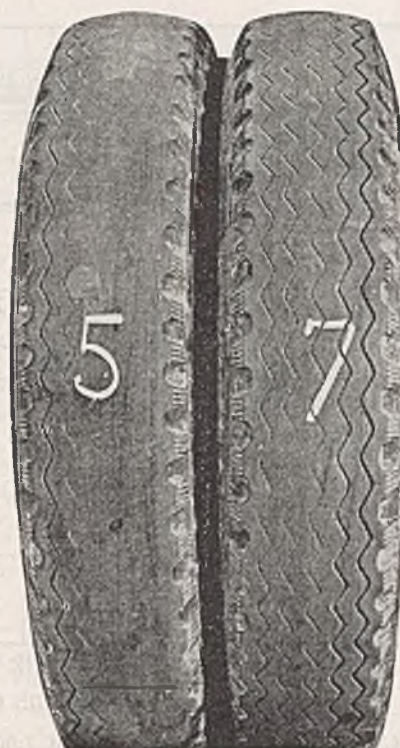
Figure 5. GR-S Tires with Natural Rubber Tubes (left) and Butyl Rubber Tubes (right) after 17,095 Miles
