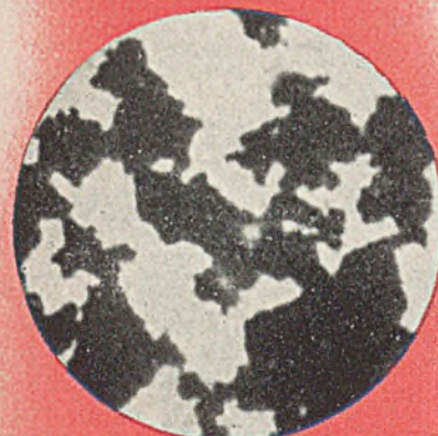
Pulverized "Barnesite" #85 (#179), magnified 5,900 times—treated until all semblance of regular particle size and shape has disappeared. Average particle size—.91 microns (about 1/25,000 of an inch). Polishing power: fast, clean, consistently so.
