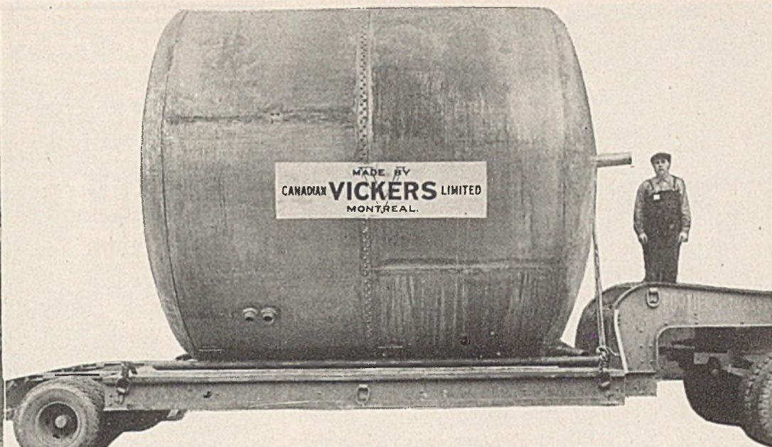
10,000 gal. capacity copper kettle, or doubler. Anaconda Cold Rolled Deoxidized Copper was used—shell and head 3/16 " thick, bottom 1/4 " thick. Internal heating unit was made from 3 " x 0.134 " copper coil, for Distillers Corporation Limited, Ville LaSalle, Quebec.
