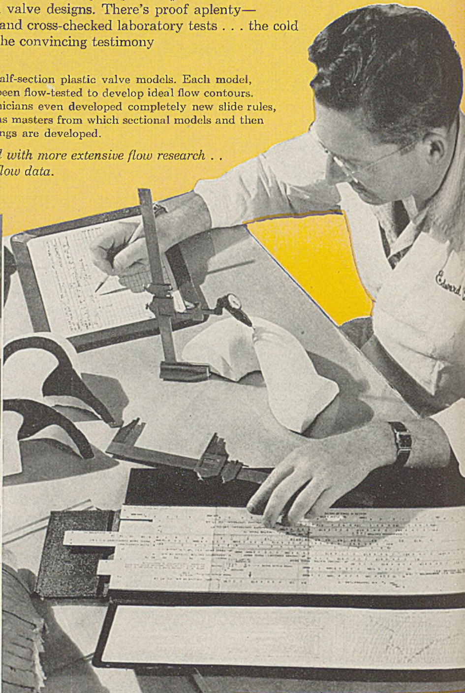
Half section super-streamlined Edward globe valve of plastic is used in flow tests. After ideal contours for high volume and minimum turbulence are established, casts are made of flow passages.
