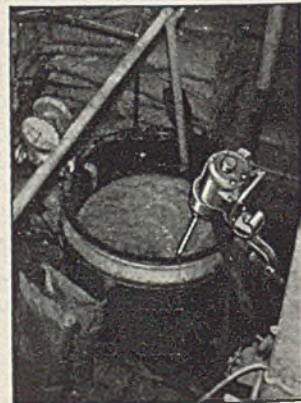
Showing how easy it is to make any tank a mixing tank.
