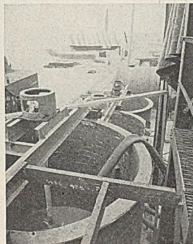
PHOSPHORIC ACID—Lead covered Turbo-Mixers in strong acid leach tanks with Atlas Mineral Products' "Rexbon" brick lining.
