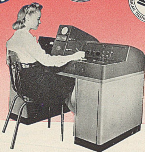
"Console" model: magnification 500 X and 5000 X; useful photographic enlargement to 100,000 diameters.
