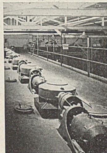
SYNTHETIC LEATHER—Battery of Turbo Nitro-Cotton Dissolvers preparing the synthetic leather base.
