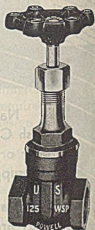
Fig. 500—125-pound Bronze Gate Valve with screwed ends, inside screw rising stem, screwed-in bonnet and either taper wedge solid or double disc.
