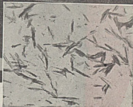
Vat Green Dyestuff X20,000—Crystal size and shape are important properties in determining suitable dyeing applications.
