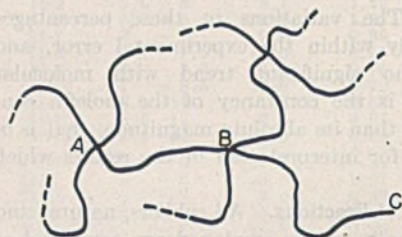
Figure 2. Diagrammatic Representation of a Portion of the Network Structure, Showing Principal Chains AB and a Terminal Chain BC
