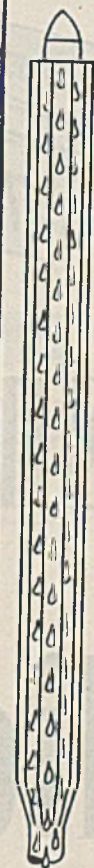
Condensate falling over vertical G-Fin tubes in constant contact with entire length of pipe
