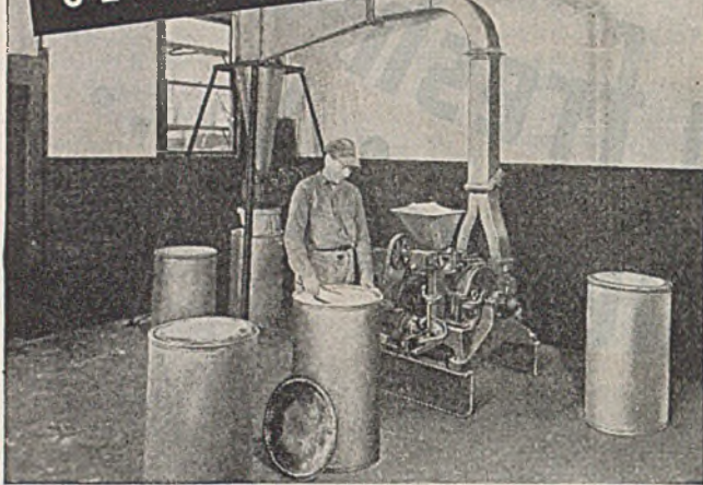
A typical No. 6 MIKRO-ATOMIZER installation. For large production operation.
