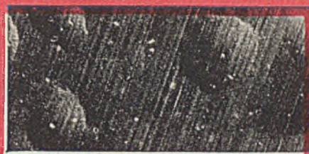
A polished face of a diamond 7,700 X—Note residual polish marks and pits in elevations.*
