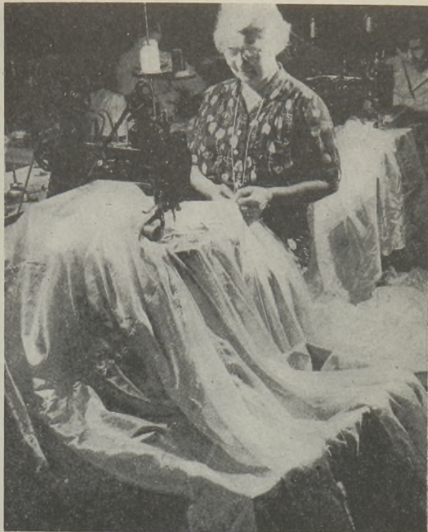
Sewing a nylon flare parachute is a joining operation in which sixteen panels, or gores, are sewn together.
