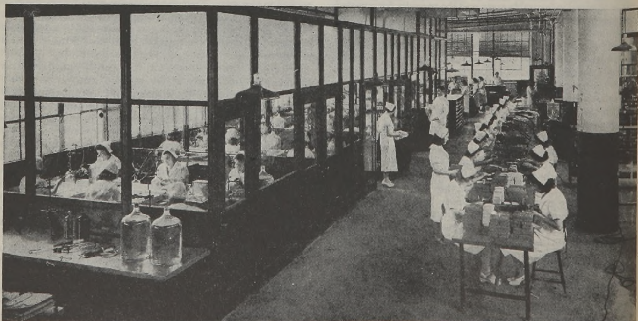
Production Department Where Solutions Are Prepared, Cartridge Glass Is Processed, Rubber Diaphragms and Plungers Are Made Ready, and Cartridges Are Filled and Packed for Shipment
