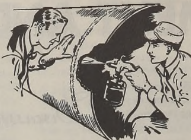
Figure 2. Testing the Porosity of a Welded Seam with an Organic Liquid
