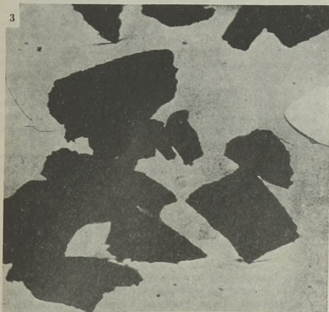
Figure 4. Scoured Wool Coated with 4% Aqueous Polystyrene Dispersion ( \times 10,000 )
