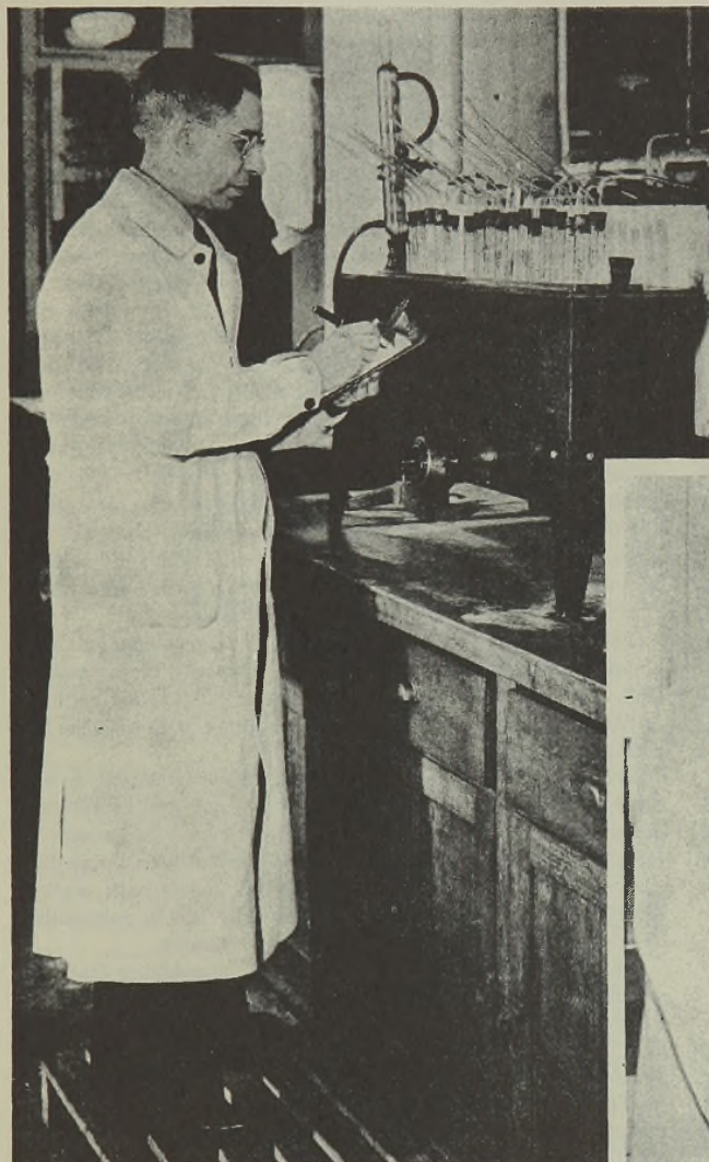
The Investigator at the Left is Working on the Determination of Keeping Quality (Rancidity) in Food Fats by the Active Oxygen Method. Below, Flavor Reversion in Soybean Oil Is Being Tested by the Only Satisfactory Test Now Known—Organoleptic.
