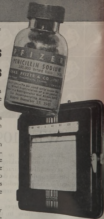
Close-up of Micromax Recorder on panel shown above. Micromax Recorders are used in the Pfizer plant to report on temperature, pH, and vacuum during the manufacture of penicillin.
