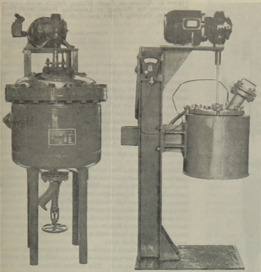
Figure 1. Integral Unit for High-Pressure Pilot Plant Work, Equipped with Agitator and Special Valve
