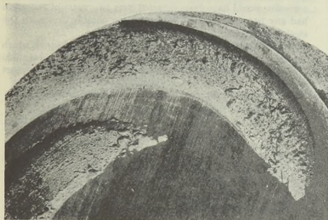
Cavitation Corrosion of a 12-Chrome Stainless Steel Impeller after Four Months of Service in Anhydrous Hydrofluoric Acid
