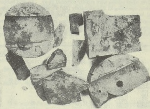
Cracking of Hardened Steel in Anhydrous Hydrofluoric Acid; These Pieces Are the Fragments of a Valve Plug
