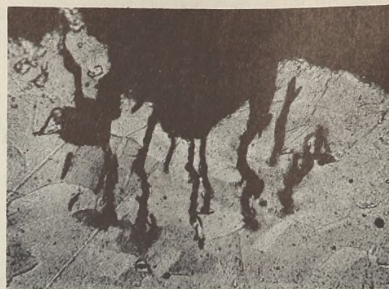
Peculiar Pitting Accompanying Denickelization of Monel by Aerated Aqueous Hydrofluoric Acid ( \times 200 )
