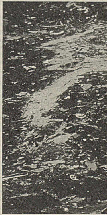
FIGURE 5. THIN CROSS SECTION OF TYPICAL SPLINT, SHOWING A HIGH CONCENTRATION OF OPAQUE MATERIAL AND FRAGMENTED REMAINS OF WOODY TISSUES (X 200)
