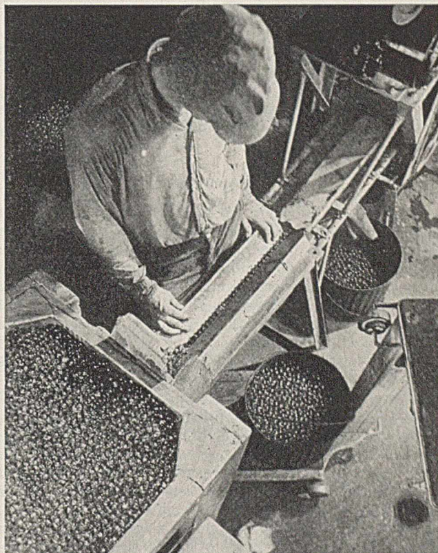
CAREFUL INSPECTION OF EACH PURE REFINED GLASS "MARBLE", THE RAW MATERIAL USED IN THE MANUFACTURE OF FIBERGLAS TEXTILES
