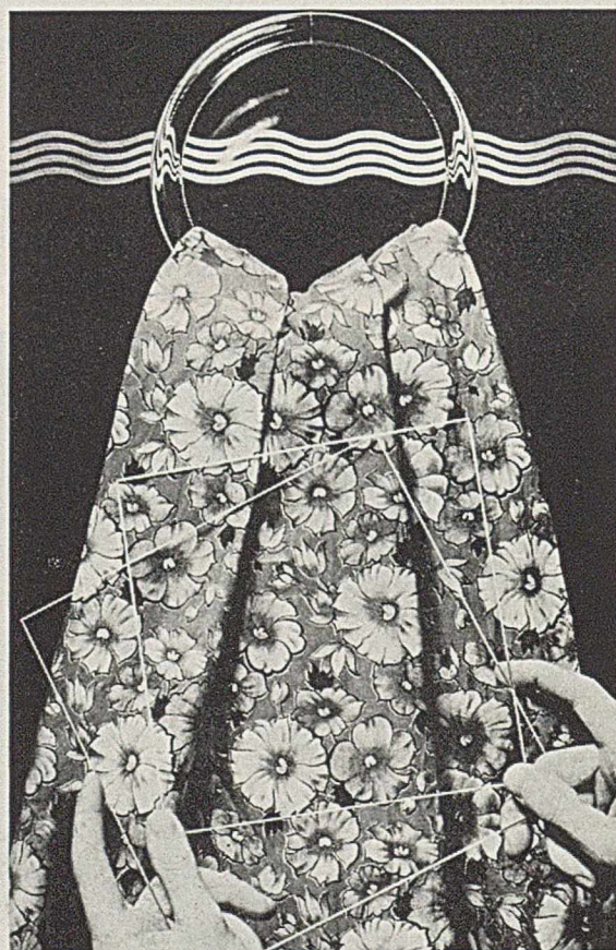
TWO SHEETS OF ACRYLATE RESIN PLACED IN FRONT OF A FABRIC TO INDICATE THE CRYSTAL CLARITY OF THIS TYPE OF RESIN
