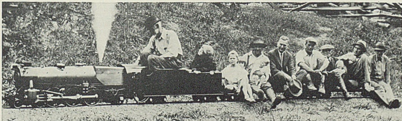
Miniature locomotive, operated as a hobby on one mile of track on an estate in Virginia, weighs 950 pounds and has tractive effort of 250 pounds, or sufficient to pull a load of 5 tons up a 3 per cent grade
