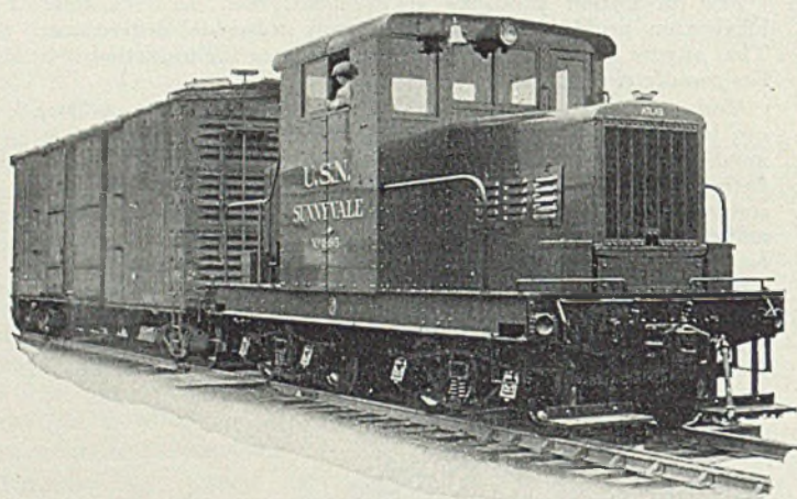
45 Ton Locomotive especially suitable for economical interplant switching service.
