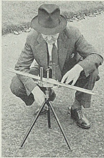
Pipelines buried 7 feet deep have been located by this magnetic detector
