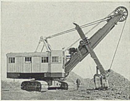
Complete one-man control features Ward Leonard excavator
