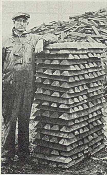
The pig has a smaller cross sectional area and weighs 40 pounds
