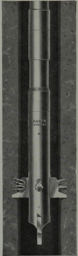
Core-taking completed—ready to bring cores to surface.
