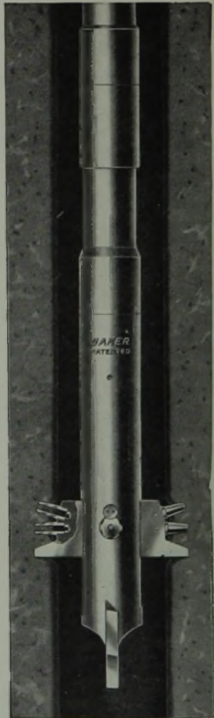
Core-taking completed—ready to bring cores to surface.
