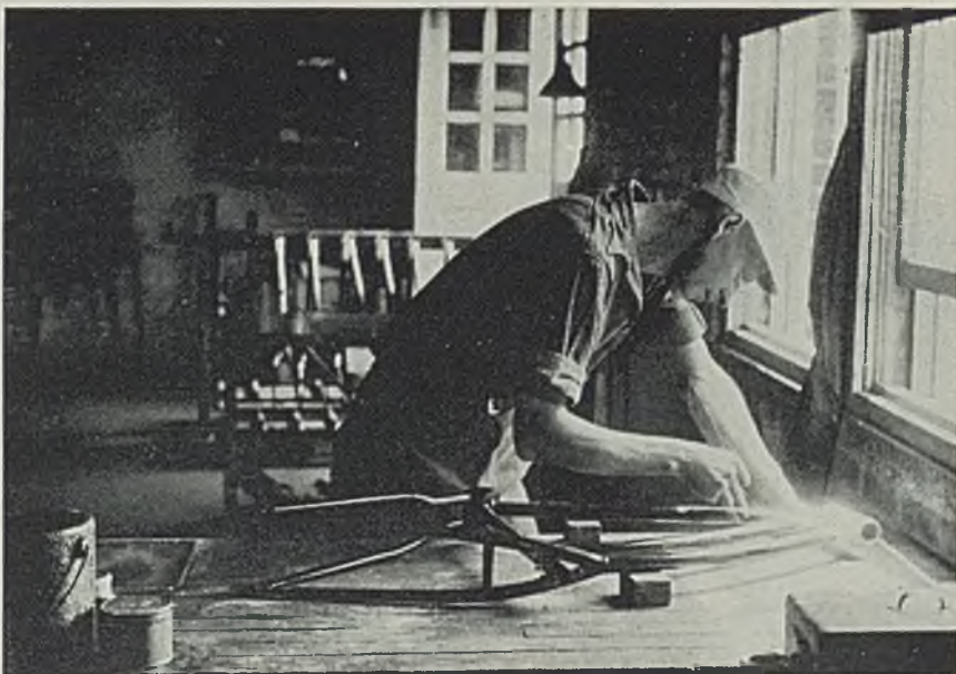
Striping of bicycle frames can only be done by hand. A high degree of skill is required for this operation as nothing will detract more from an otherwise excellent finish than poor striping
