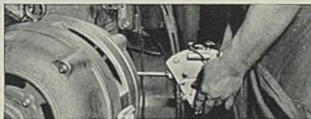
Every motor is given a thorough vibrometer test to make sure proper dynamic balance. Eliminate vibration and you reduce to a minimum the wear on bearings. Sealed ball bearings and smooth running insure trouble-free service from F-M motors under the severest operating conditions.
