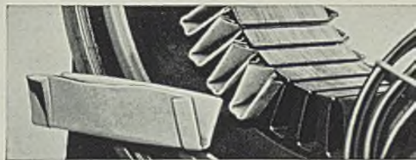
Special cuff insulation. Empire cloth inside of two special formed fibrous sheets is inserted in the stator core slots. A genius method of folding makes a self-locking cuff which gives permanent protection to the coil when it leaves the stator slot.
