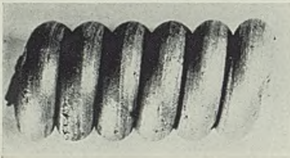
FIG. 6 — Breaks shown in this bent wire are a direct result of imperfections shown in illustrations above
