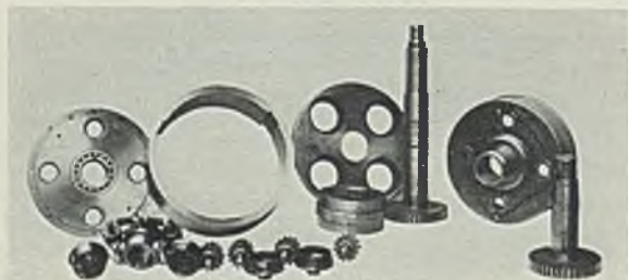
Dissembled parts of the automatic gear change unit, showing simplicity of construction. If required, more gears may be added to increase the ratio
