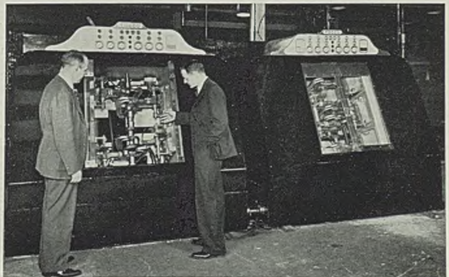
M. A. Tran (left) and W. E. Benninghoff demonstrate features of the machine, they have developed for surface hardening of automotive crankshafts by induction heating, the equipment being exhibited in operation at the exposition
