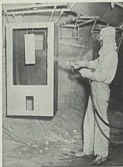
Suitable surface conditions permit continuous finishing of assembled cabinets, affording appreciable reductions in manufacturing cost
