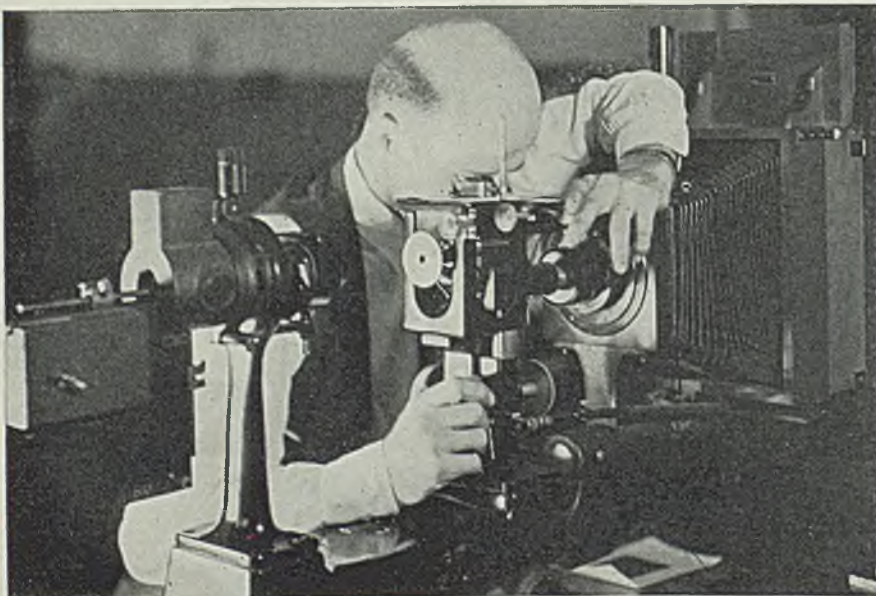
With this type of metallographic apparatus the test pieces can be examined visually or photographed for future reference
