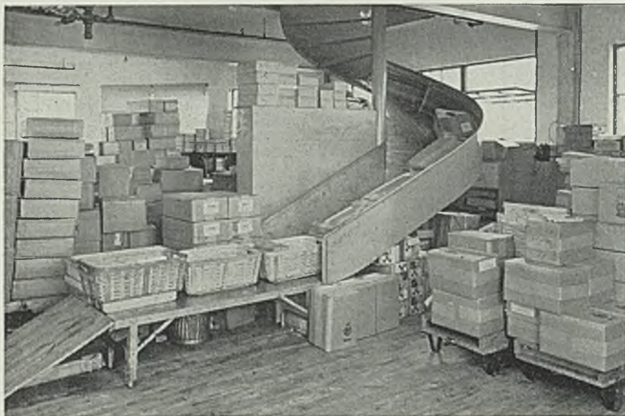
FIG. 2—View of section of shipping department showing delivery end of spiral chute which connects with the manufacturing building. A gravity roller conveyor also is used for handling outgoing shipments
