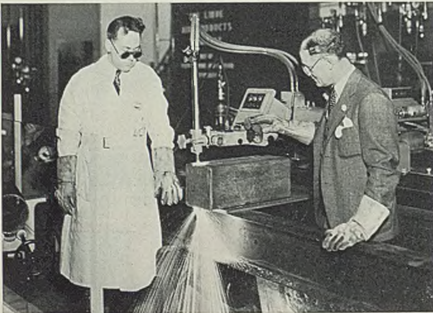
O PERATOR S. R. OLDHAM (left) demonstrates to A. E. Gibson, new president of the American Welding Society and vice president, Wellman Engineering Co., something new in automatic shape cutting machines at the metal show in Cleveland. The machine, part of the exhibit of Linde Air Products Co., is slicing a 10-inch steel billet
