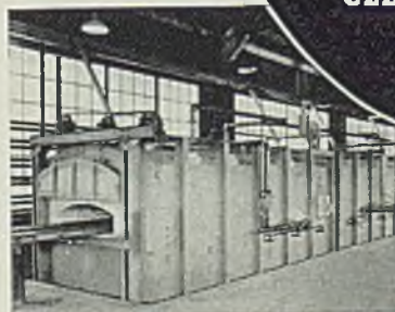
Pusher Type Normalizing Furnace for Rear Axles
