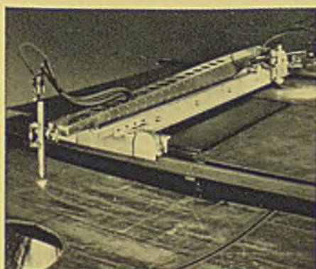
The Oxweld CM-11 (100-inch) cutting a machine frame member from a 2-inch steel plate 8 feet square.
