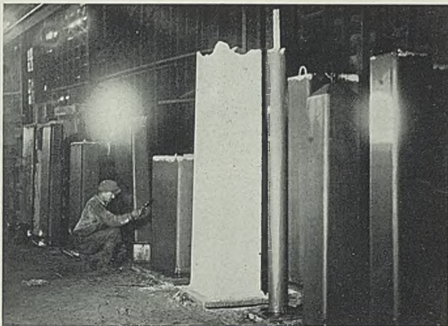
Painting of finished cores for ingot molds. After painting they are allowed to set for one to three days
