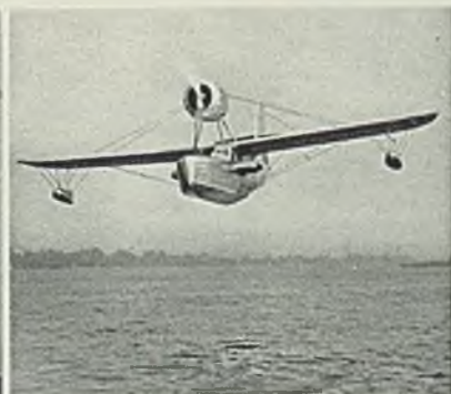
THE FLEETWINGS' "Sea Bird" amphibian is stronger, safer, and over 200 lbs. lighter than equivalent planes of conventional construction. USS Stainless Steel was specified for every part except motor and wing covers.
