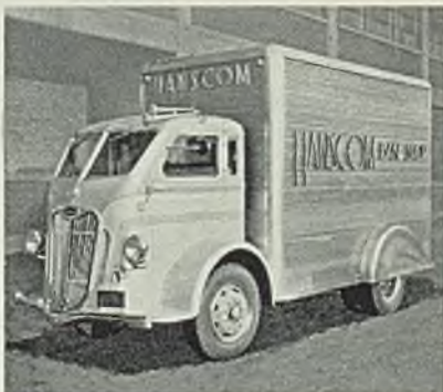
THREE BIRDS with one stone . . . This smart New York bakery truck of gleaming stainless steel saves weight, reflects heat, makes a most effective advertisement.
